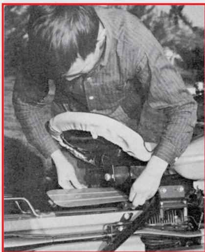
A plate lifts from the rear deck to permit adjustments to clutch and transmission. Note the rubber seat mount above the plate.
