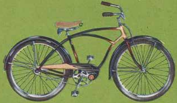
The Schwinn Standard Autocycle . . . The ideal bike for those who desire the added advantages of the patented cantilever frame construction without the special equipment. Included are chainguard, built-in kickstand. 26 inch model No. B-4.
